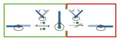
An open-and-closed case: When a chiral clamp is attached to a molecular hinge the open—close motion induced by coordination to a metal ion becomes unidirectional (see scheme). The large change in ampli-
