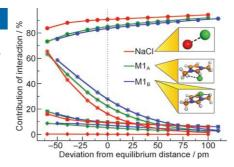
A subtle difference: In ionic liquids the "weak" dispersion forces have a significant impact on the shape of the potential energy surface, which results in a shallow profile when all of the contributions are considered. Such findings are commonly accepted to determine the liquid state.
