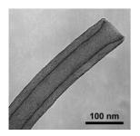
Controlled growth: A non-aqueous approach inspired from sol-gel chemistry and adapted to the formation of metal oxide thin films by means of atomic layer deposition is presented. The process is based on the reaction of a carboxylic acid with an alkoxide. Growth of metal oxides is achieved at temperatures as low as 50 °C on various supports including carbon nanotubes (see TEM picture). The as-grown films show excellent uniformity and possess good dielectric properties.
