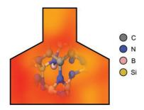
An unlikely couple: Carbon and nitrogen usually go separate ways above 600°C, but in a precursor-derived high-performance SiBNC ceramic pyrolyzed at 1400°C the presence of carbon–nitrogen bonds was demonstrated by using various double-resonance solid-state NMR techniques in combination with a novel isotope labeling scheme.
